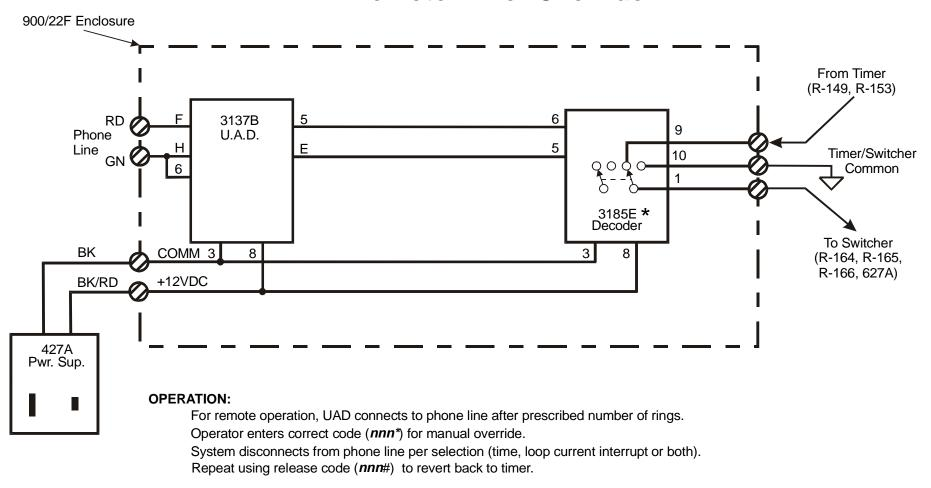
**NOTE\*** Only one set of contacts are shown connected. Additional NO and NC contacts are available on the 3185E card for other uses.
